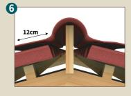
Use a ridge batten to support the Onduline ridge piece as shown. The ridge element has to overlap the ONDULINE® sheet minimum 12 cm.
