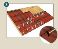
The fixing on each corrugation should be done in the right order and in between the 2 overlapping guides. Do not fix those corrugations that will be overlapped by the next tile or verge piece.
