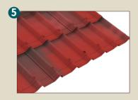
If the opposite end the roof doesn't finish with a corrugation, cut the last tile at the edge of the roof and use a batten as a support for the corrugation. Bend the last tile over the batten, in order to ensure proper waterproofing.
