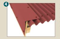
Optimize aesthetic, waterproofing, and wind uplift resistance by using a verge element. Fix it first into the sidewall, then on the top of the corrugation.
