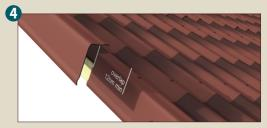
The aesthetics and wind uplift protection can be optimized by using the verge element accessory, which is fixed first on the sidewall, then as well on the top of the corrugation. Plan 6 fixings per elements.
