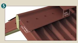
Cover the ridge and fix it on each side of the roof, on top of each corrugation. The direction of the overlap is opposite to the direction of the prevailing winds.
