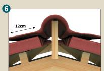
Use a ridge batten to support the Onduline ridge piece as shown.
