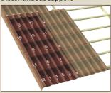
15 fixings minimum should be used per sheet. The fixing, always set in the top of corrugations on the grey marks, should be done in the right order. Wait to fix the last corrugation until you overlap it with the verge element or the next sheet.
