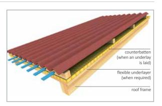
A1 = A2 = Distributed ventilation inlets and outlets needed (in cm2) : Ventilation openings A1 and A2 should be provided at each eave and at the roof ridge (see figure B). If the roof pitches are longer than 20 meters, an extra opening should be included at an intermediate point on the pitch. Refer to the following chart to determine the ventilation needs especially for low pitches less than 15°.
