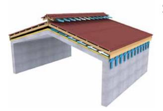
Narrow buildings with high pitched roofs are better ventilated when compared with wide buildings with lowpitched roofs. That is why the horizontal distance between the eaves and ridges and the roof inclination must be taken into consideration when determining the space necessary for ventilation.
