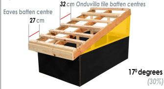
Onduvilla tile strips can be laid on a purlins with a minimum batten width of 50 mm and 25 mm depth in conformity with relevant British Standards and Codes of Practice.
