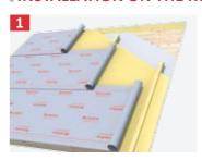
Roll out ONDUTISS® AIR in parallel with the gutter, starting from the bottom, always the printed side facing up. The membrane can be laid directly on the thermal insulation with slight tension. The overlap is indicated by lines or logo print. For the highest water tightness seal ONDUTISS® AIR bands with ONDUTISS® sealing tape.
