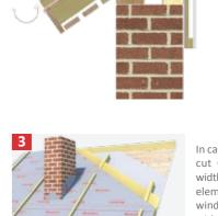
In case of any protruding element, cut ONDUTISS® AIR across the width and turn up on the protruding elements (chimneys, ventilations, windows etc.). Fix ONDUTISS® AIR with ONDUTISS® sealing tape. NB! Please, check the detailed
