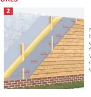
Fix ONDUTISS® AIR bands with battens/ framing structure. Install external cladding elements (siding, facade panels, steel plates etc.). Ventilation gap between ONDUTISS® AIR and the external cladding should be at least 3 cm.
