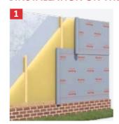
Roll out ONDUTISS® AIR parallel to the floor, starting from the bottom so that natural release of condensation would be possible. The printed side should always be face up. ONDUTISS® AIR can be laid directly on the thermal insulation. The overlap is indicated by lines or logo print. Fix the bands directly to the frame with a stapler. All the joints should be sealed with ONDUTISS® sealing tape.
