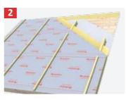
Fix the bands directly to the rafters with a stapler. Nail counter batten on top of the membrane through to the rafters to protect the fixing area.
