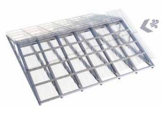
Install the sheets from the eaves to the ridge, starting from the opposite direction of prevailing winds.
