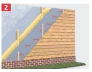
Fix ONDUTISS® Wind 100 bands with counter battens/ framing structure. Install external cladding elements (siding, facade panels, steel plates etc.). Ventilation gap between ONDUTISS® Wind 100 and the external cladding should be at least
