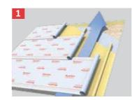
Roll out ONDUTISS® CROSS 80 vapour proof membrane across the rafters starting from the bottom. Ventilation gap between the ONDUTISS® CROSS and insulation should be at least 2 cm. The overlap should be at least 10 cm.
