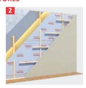
Fix ONDUTISS® BARRIER bands in place by applying the supporting structure of the interior paneling. Ventilation gap between the membrane and the interior paneling should be at least 3 cm.
