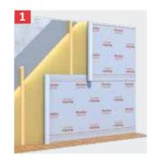
Roll out ONDUTISS® BARRIER vapour proof membrane in parallel to the floor always the printed side facing you. The overlap is indicated by lines or logo print. Fix ONDUTISS® BARRIER bands directly to the frame with a stapler. Use ONDUTISS® sealing tape to seal all joints and connections.
