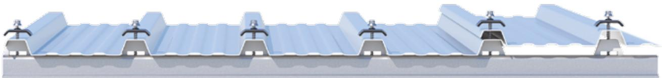
Main fasteners are always located on the top of each rib (corrugation) and on each support (purlin).
