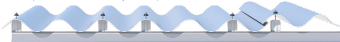
Fasteners are located on the top of the 1<sup>st</sup>, 3<sup>rd</sup>, 4<sup>th</sup> and 6<sup>th</sup> corrugations.
