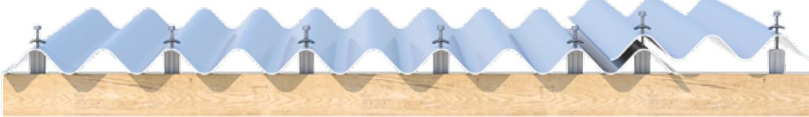
One fastener each two corrugations at the top and the bottom of the sheet plus one fastener at sidelap.
