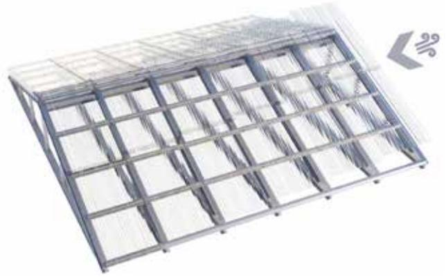
Install the sheets from the eaves to the ridge, starting from the opposite direction of prevailing winds.
