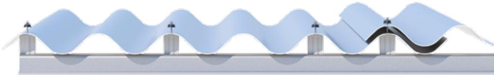
Fasteners are located on the top of the 1<sup>st</sup>, 3<sup>rd</sup> and 5<sup>th</sup> corrugations.
